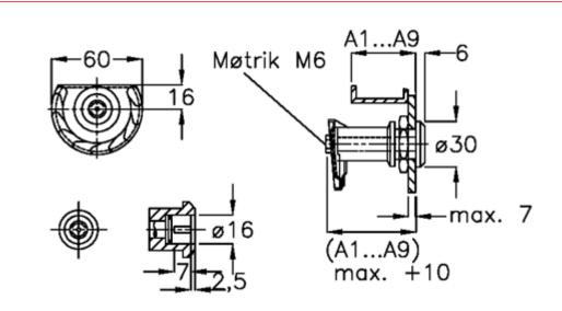
Door + frame thickness = 22-30 Measure type = A2
